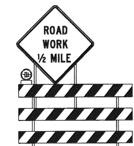
WITH TYPE "B" FLASHING WARNING LIGHT MOUNTED ABOVE TYPE III BARRICADE
