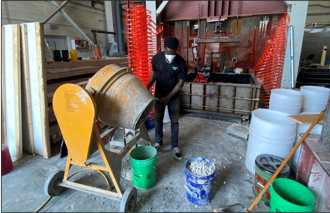
Figure 4.35 Aggregate mixing at OMC using concrete mixer
