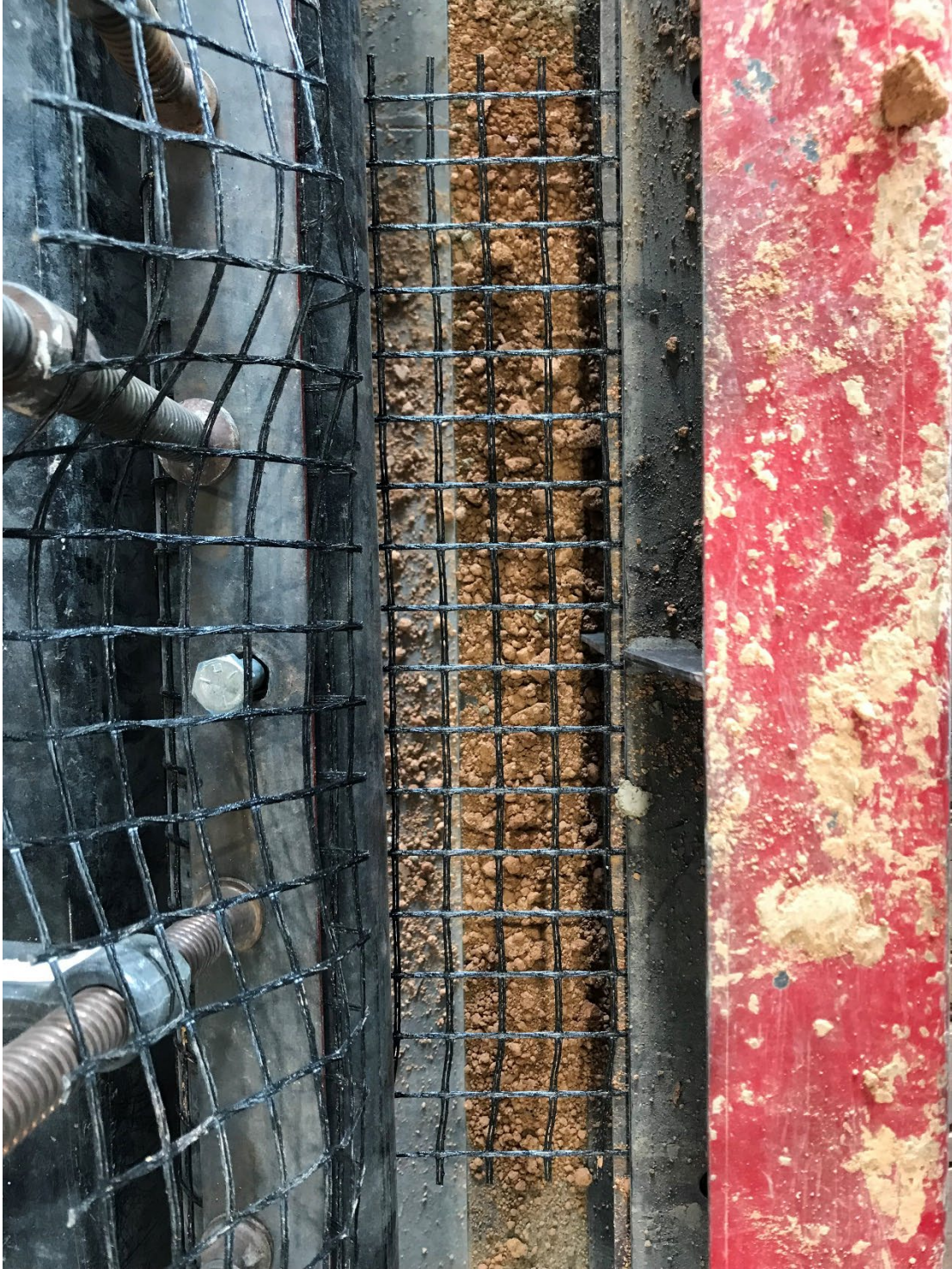
Figure B.8 Pull out of geogrid during the test
