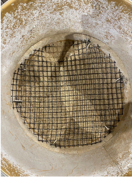
Figure 4.22 2XT (GG3) geogrid on compacted sand subgrade
