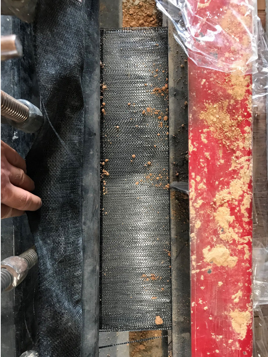
Figure B.9 Pull out of geotextile during the test
