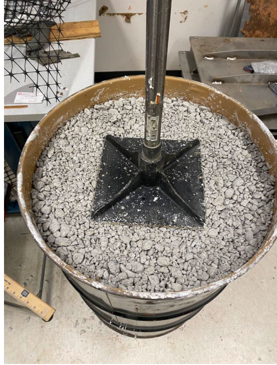
Figure 4.19 Compacted gravel base course layer
