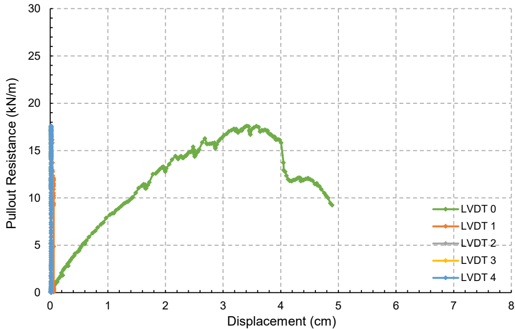
Figure 5.56 GT reinforced clay at 38 kPa
