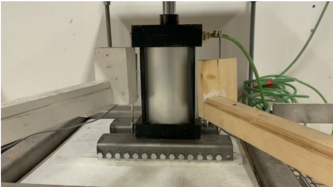
Figure 4.2 Positioning of LVDTs in the A) vertical and B) horizontal direction
