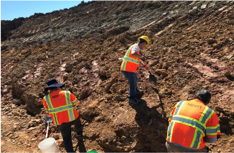
Figure 3.4 Collection of soil for testing
