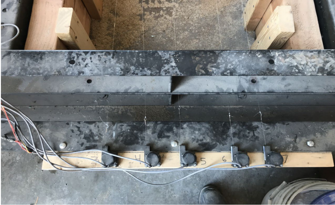
Figure 4.8 LVDTs (telltales) attached to the rear portion of the box
