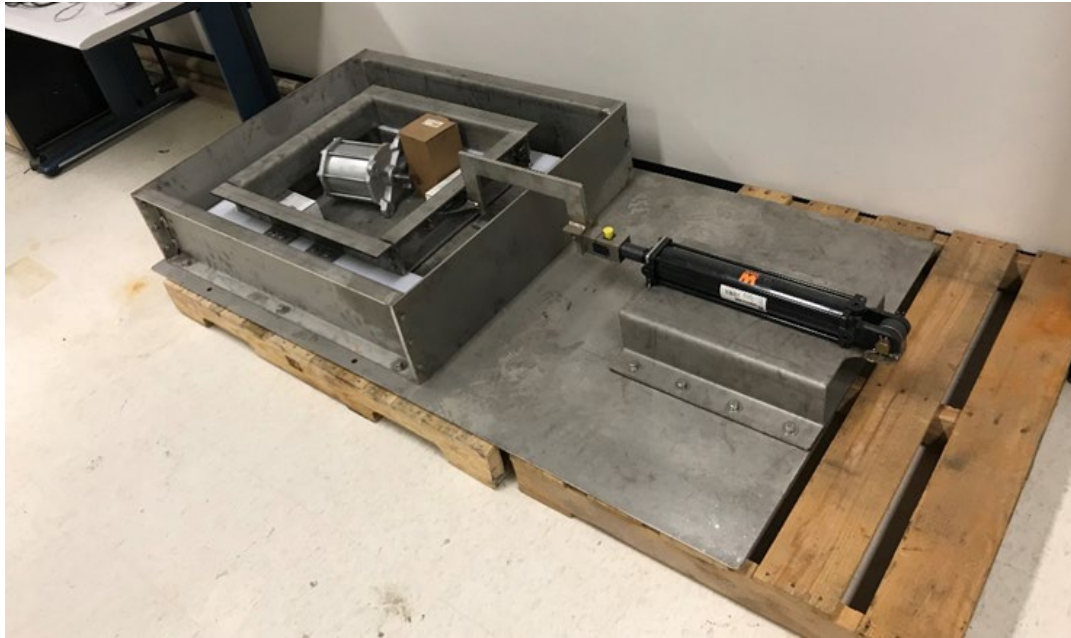
Figure 4.1 Initially fabricated direct shear apparatus
