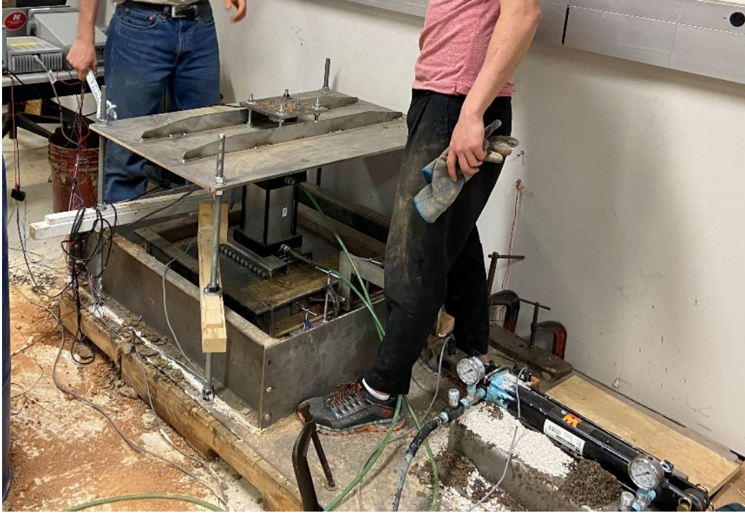
Figure A.6 A large direct shear test setup
