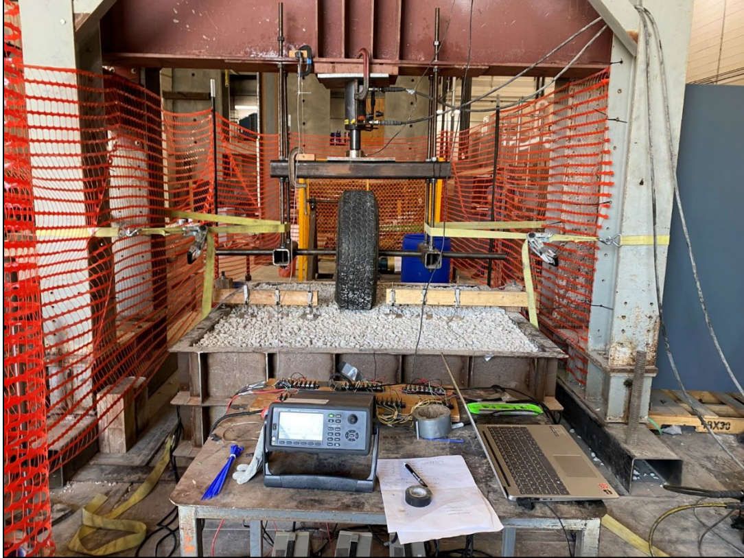
Figure 4.45 LSTW complete test setup
