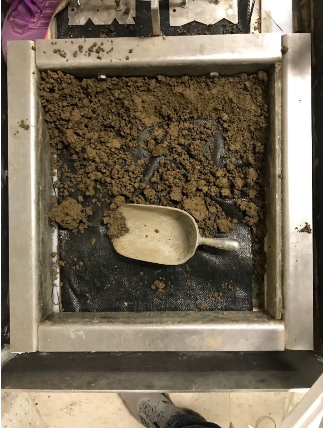
Figure A.3 Installation of geosynthetic specimen in clay
