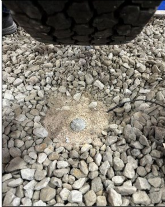
Figure 4.41 Pressure cell installed on top of base course
