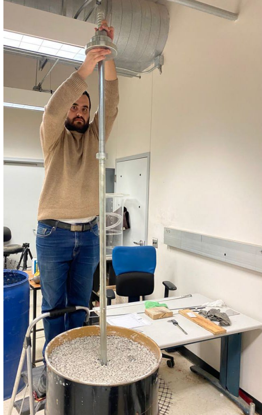
Figure 4.29 DCP test on compacted base course and sand layer
