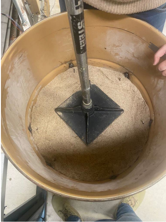
Figure 4.18 Compacted sand subgrade layer
