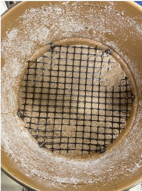
Figure 4.20 BX1200 (GG1) geogrid on compacted sand subgrade
