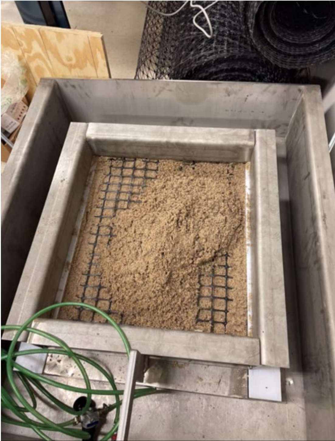
Figure A.1 Installation of geosynthetic specimen in sand
