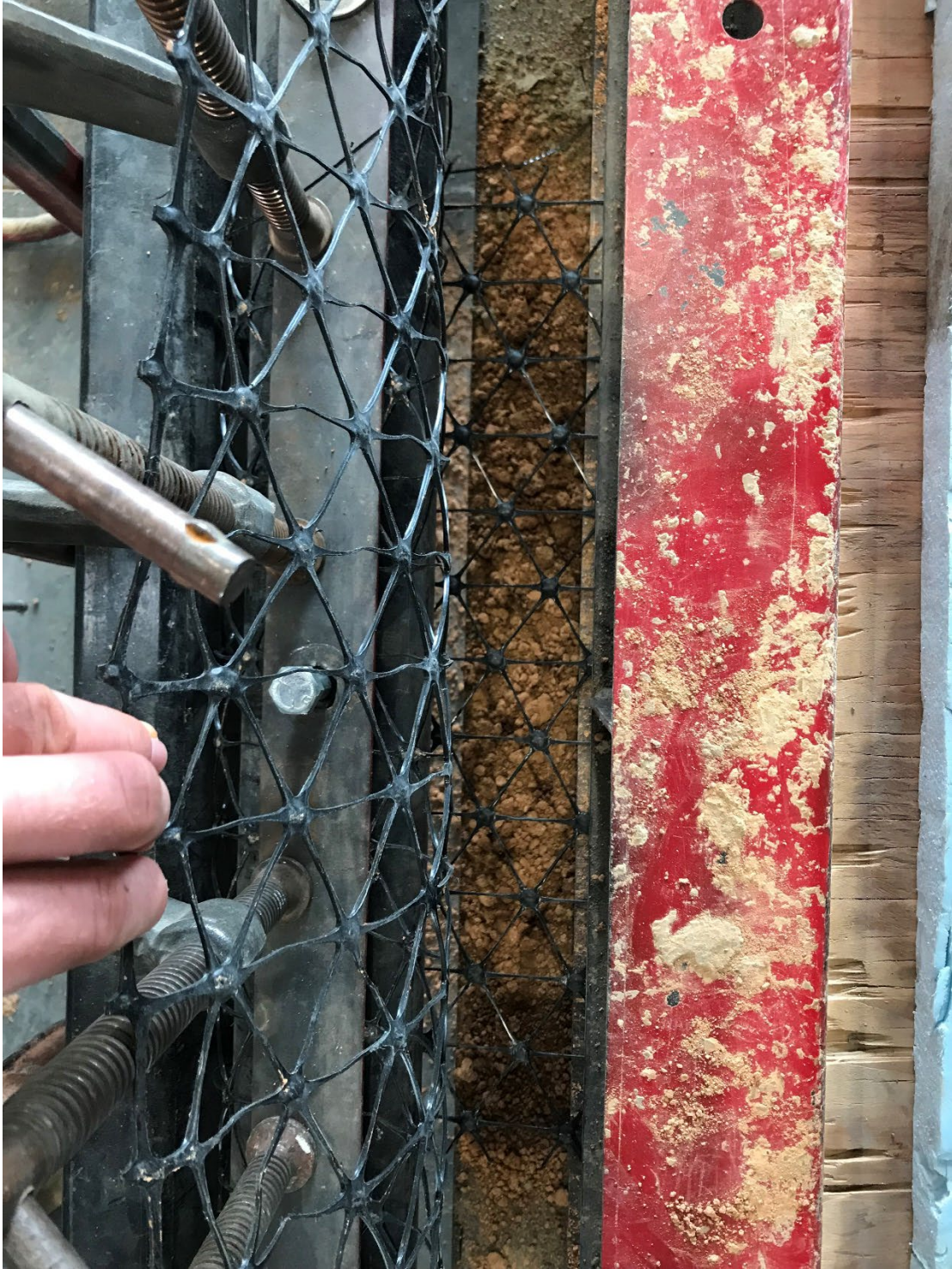
Figure B.7 Pull out of geogrid during the test
