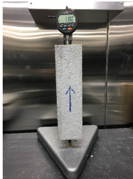
Figure 3.22 Length comparator used in the free shrinkage test
