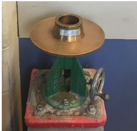
Figure 3.6 Flow table test apparatus
