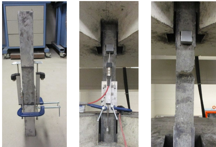
(a) specimen preparation (b) setup (c) typical failure mode
