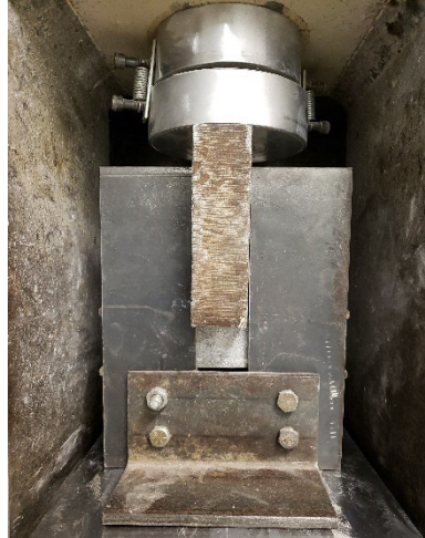
Figure 3.14 Direct shear test setup
