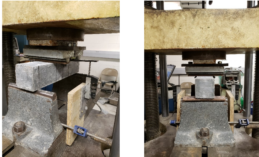
Figure 3.11 Flexure strength test setup
