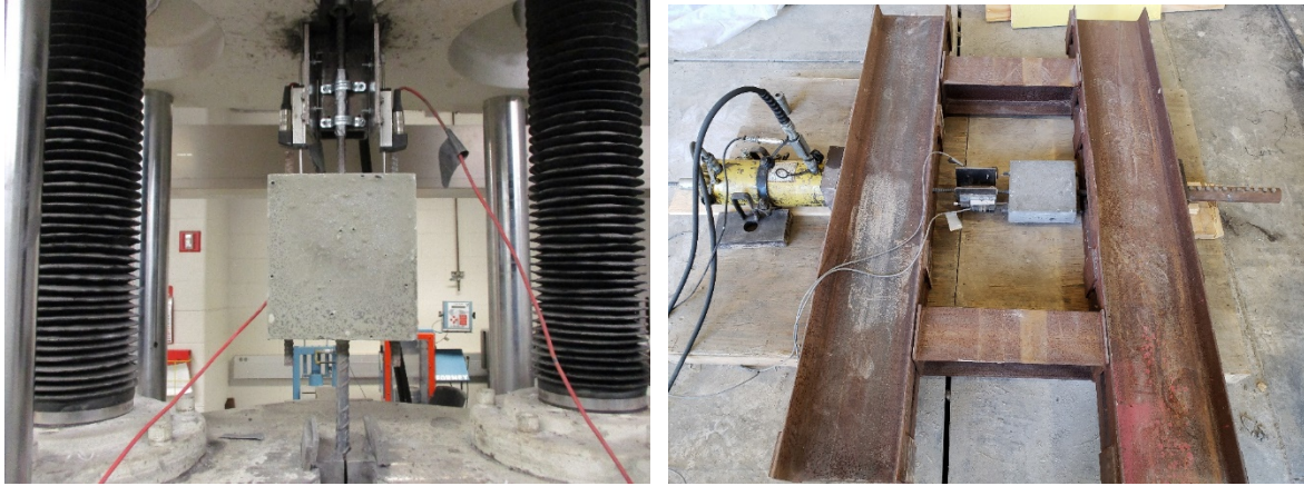
Figure 3.18 Rebar bond strength test setups
