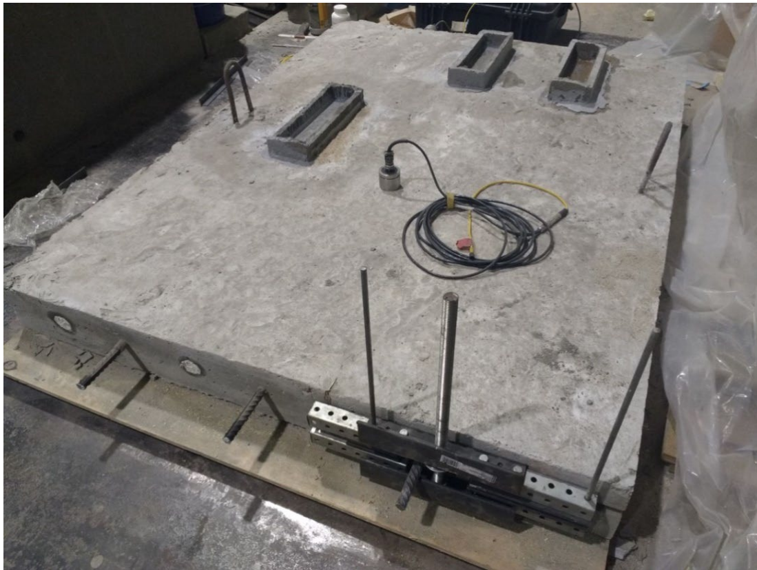
Figure 3- Specimen Set 1B (Corrosion-delamination Specimens)
