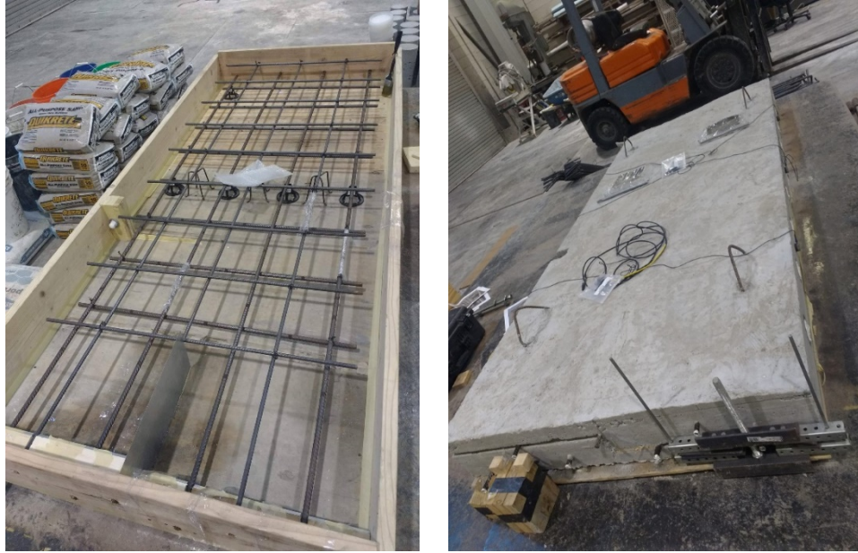
Figure 5- Specimen Set 3 formwork and bars before casting (left) and final specimen (right)
