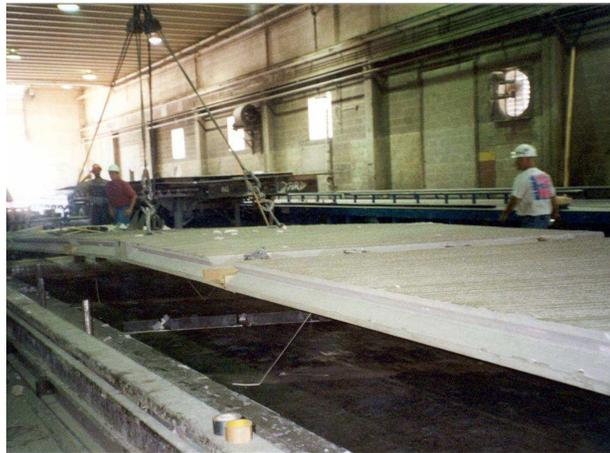
Figure 3.7-Lifting Panel out of the Prestressing Bed
