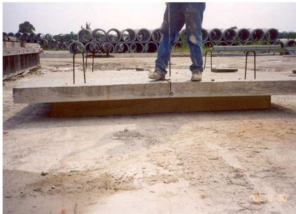
Figure 3.15-Removing the Top Steel Plate
