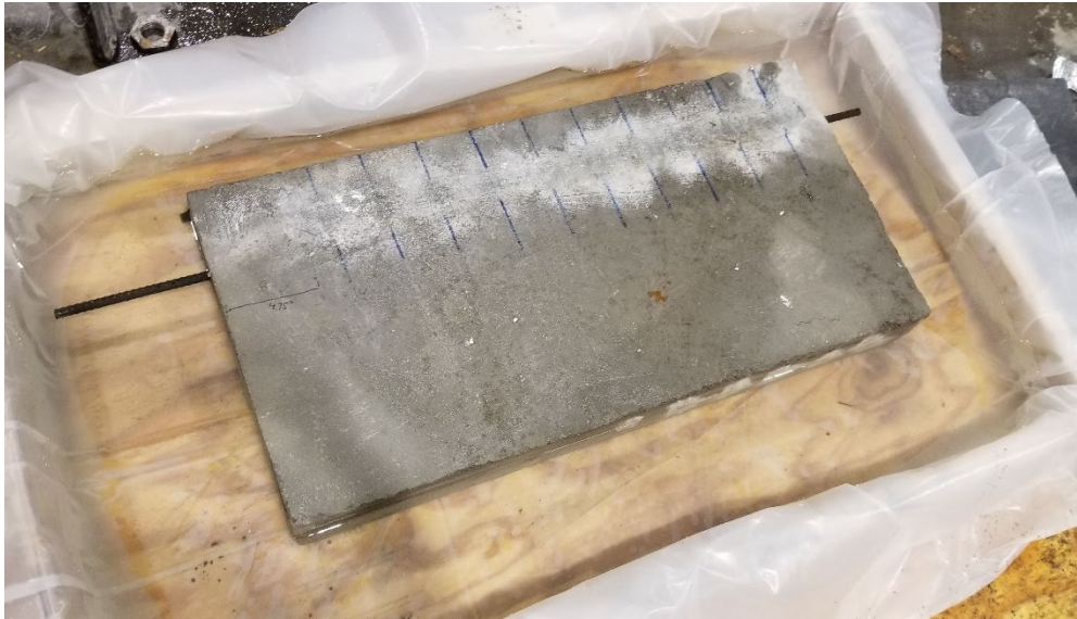
Figure 16. Test specimen submerged inside 10% NaCl solution
