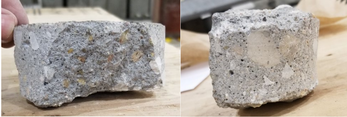
Figure 30. Extracted cores from the concrete specimen
