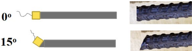
Figure 36. Bar end angles for corrosion specimens in Specimen Set 3
