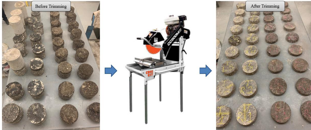
Figure 3.4 An example of PMFC specimens before and after trimming
