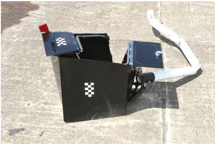
Figure 14. Locking Architectural Mailbox on Single Mount Post - Test No. 490023-9-2, Test Results
