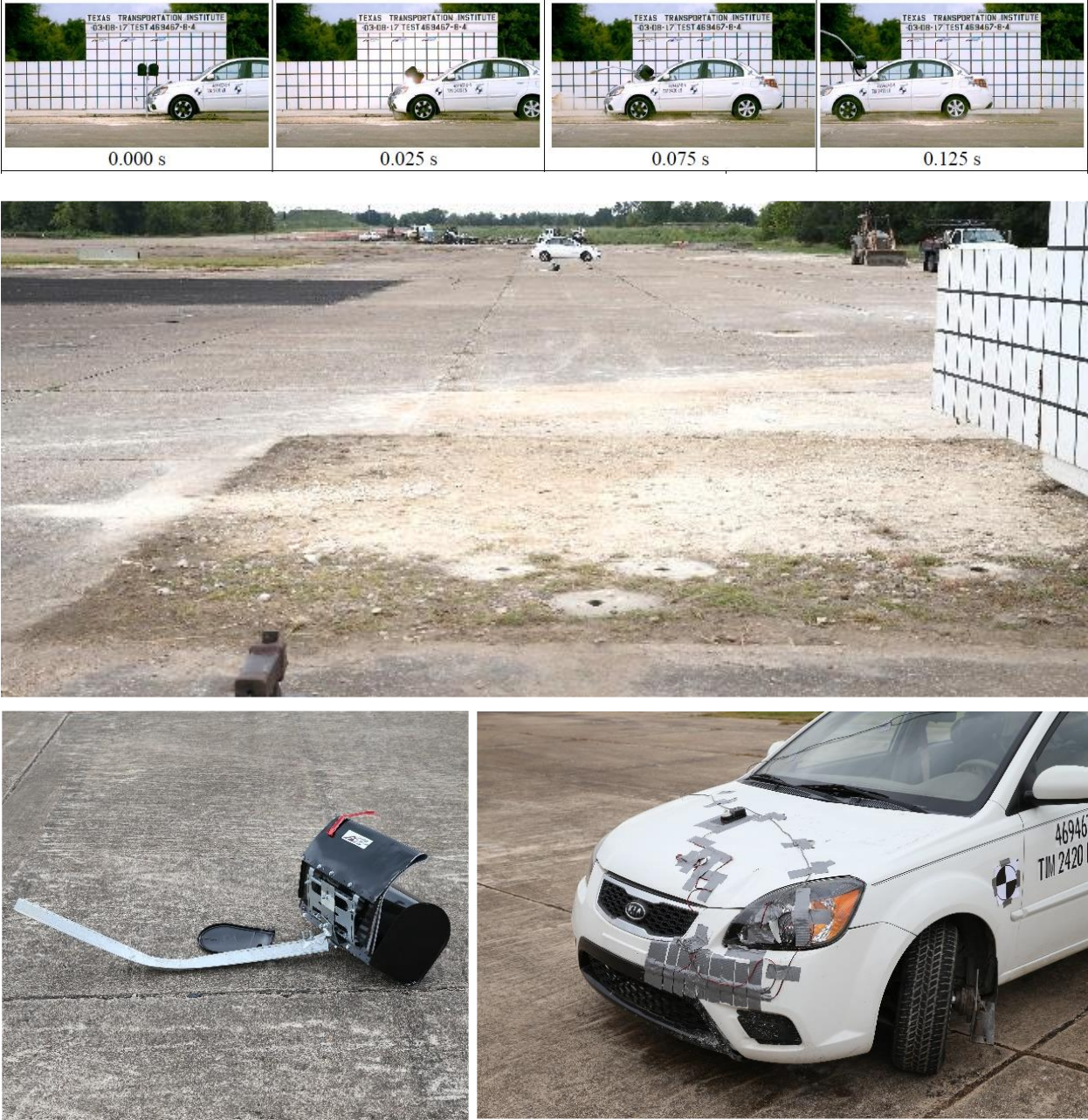
Figure 3. TxDOT Winged-Channel Mailbox Support - Test No. 469467-8-4, Test Results
