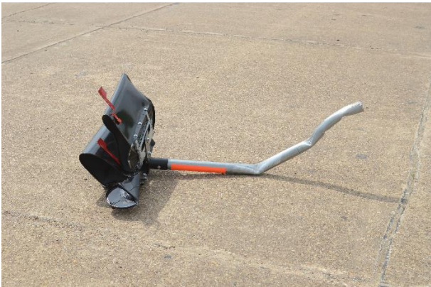
Figure 21. Double Mailbox with Thin-Wall Galvanized Support Post in Type 4 Foundation - Test No. 469468-8-2, Test Results
