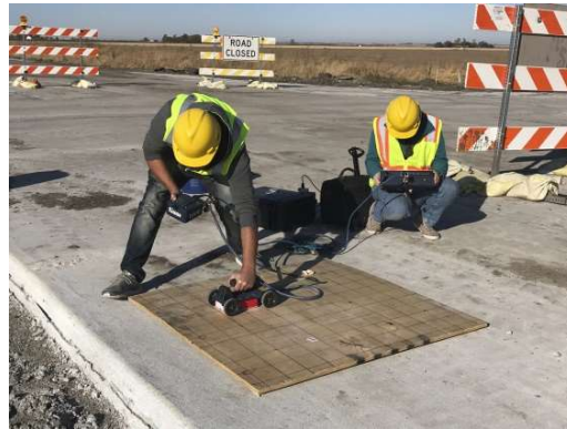
Figure 2.23 Field Experiment 2 - GPR Scanning
