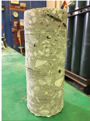
Figure 2.19 Slab 3 - Core 13 (Compressed Air)
