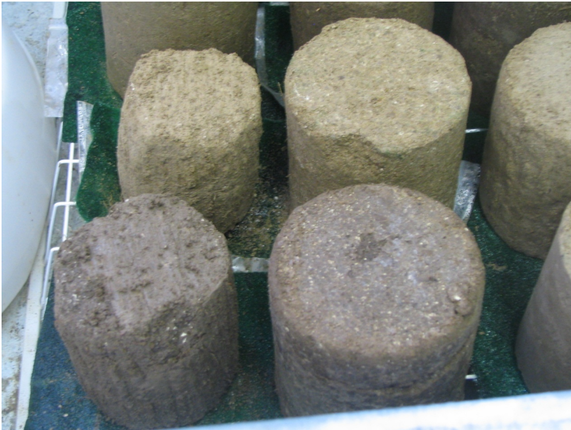
Figure 6: Freeze-Thaw Test Specimens
