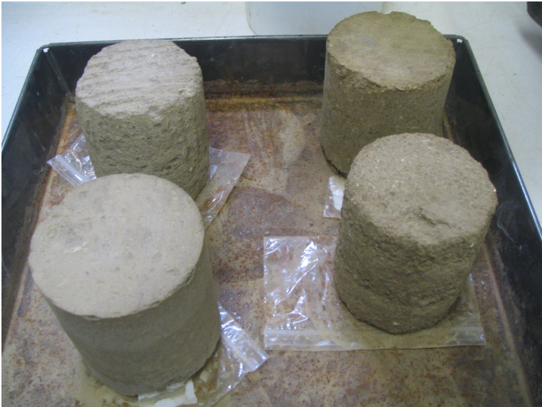
Figure 8: Wet-Dry Test Specimens
