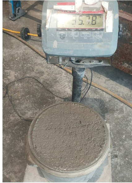
Figure 3.8 Unit weight measurement
