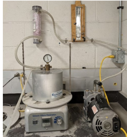
Figure 3.31 Sample preparation in vacuum saturation chamber
