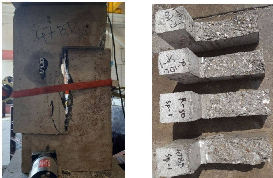
Figure 5.14 Shear failure (left) and failure plane of the specimens (right)
