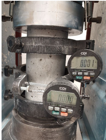
Figure 3.18 Static modulus of elasticity test setup
