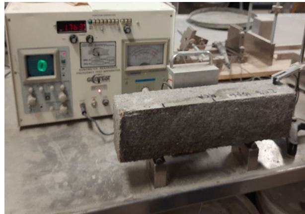
Figure 3.28 F-T resistance test setup with sonometer
