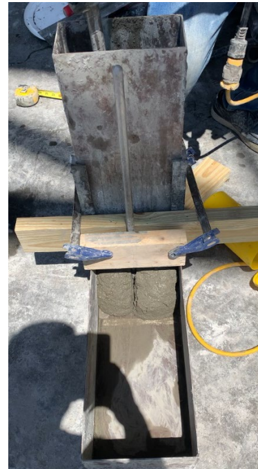
Figure 3.13 Concrete passing the 6-inch mark under vibration in L-box
