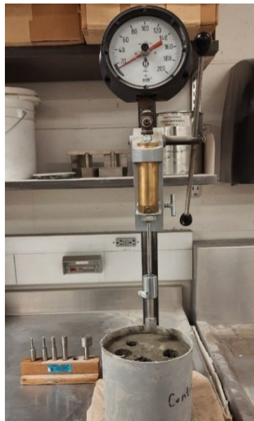
Figure 3.14 Penetration resistance test for concrete set time
