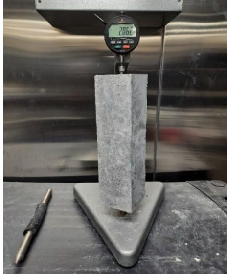
Figure 3.35 Change of concrete length measurement
