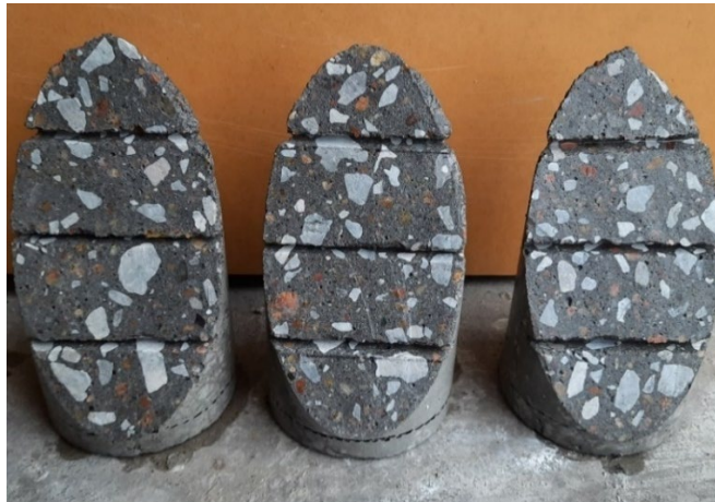
Figure 3.23 Prepared surface of old concrete (47BD)
