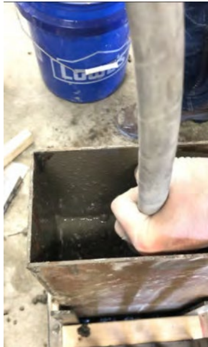
Figure 3.12 Insertion of the vibrator in L-box
