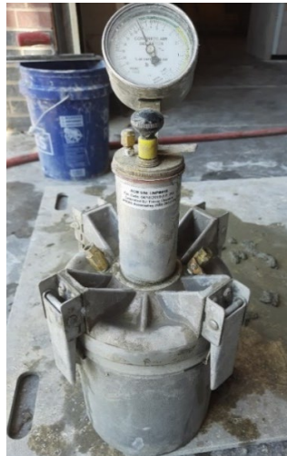
Figure 3.9 Air pressure measurement (meter type-B)
