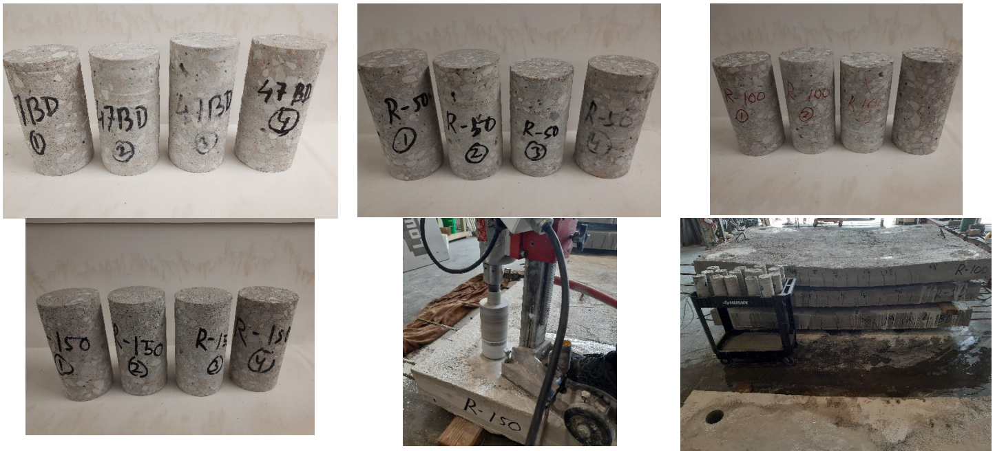
Figure 5.12 Concrete cores taken from tested slabs
