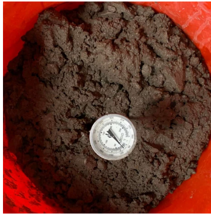
Figure 3.6 Fresh concrete temperature measurement
