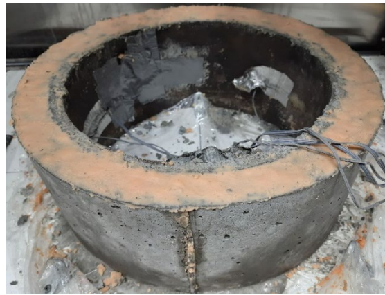
Figure 3.34 Concrete test specimen in the environmental chamber
