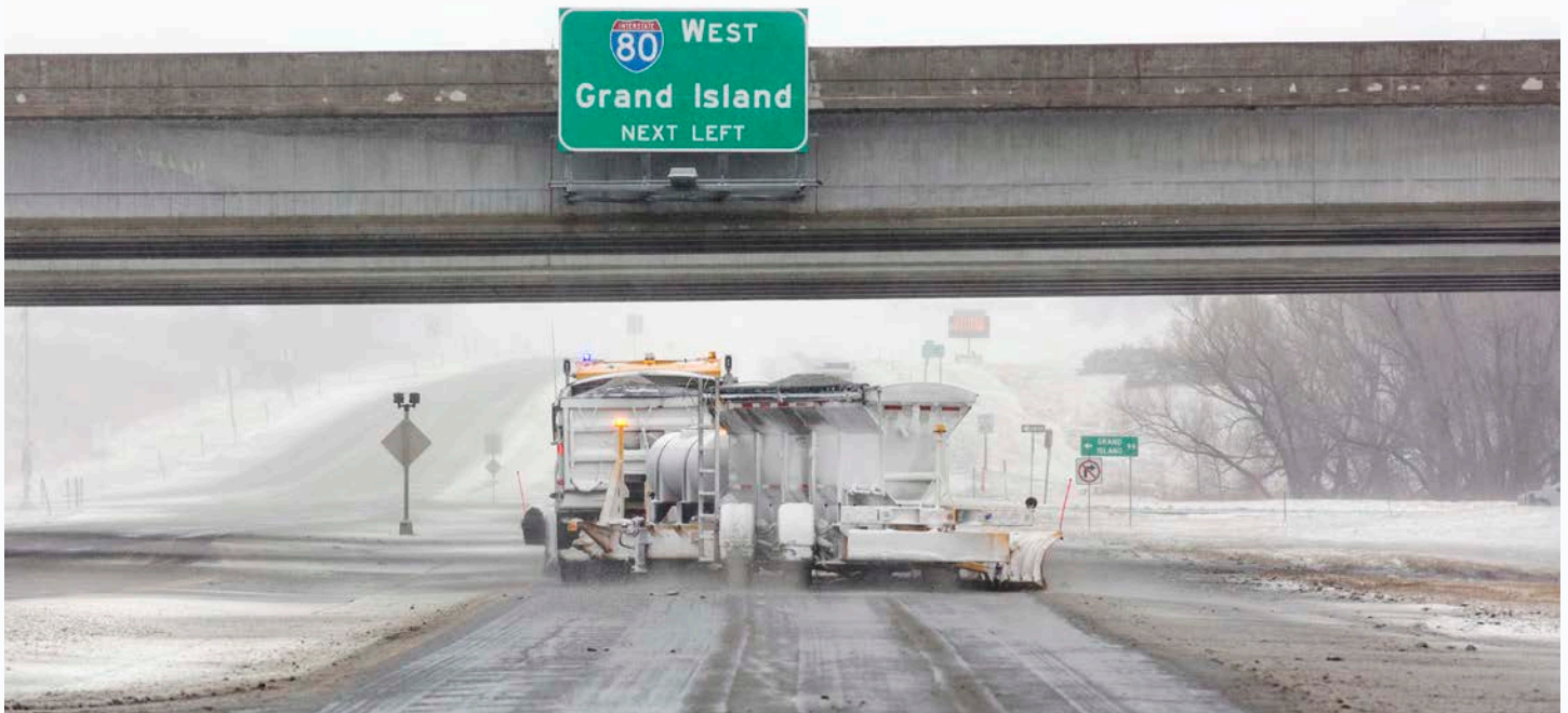
Tow plow in action east of Lincoln on US-77 near the I-80 on-ramp.
