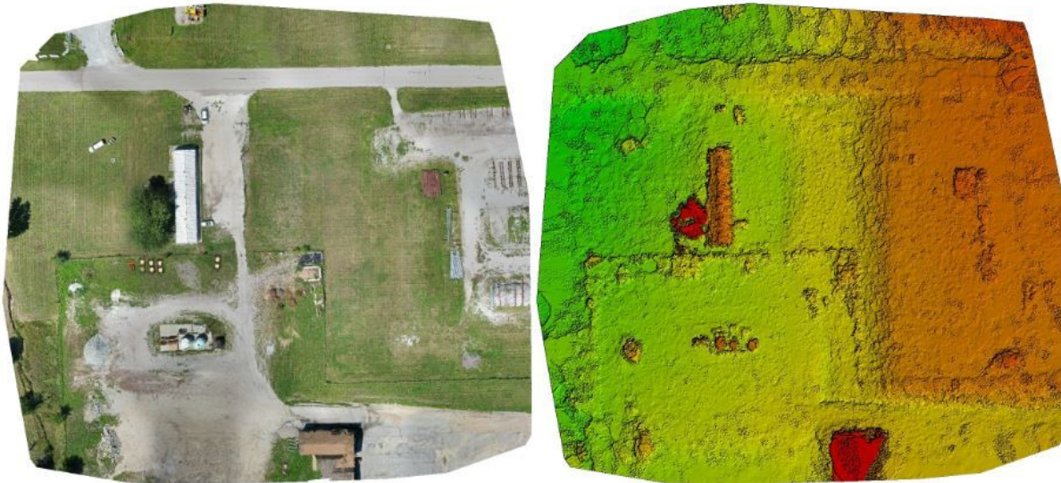
Figure 4. Color orthomosaic (left) and digital surface model (right) produced using imagery acquired during a field training flight and processed with the Pix4D software also used in the training.
