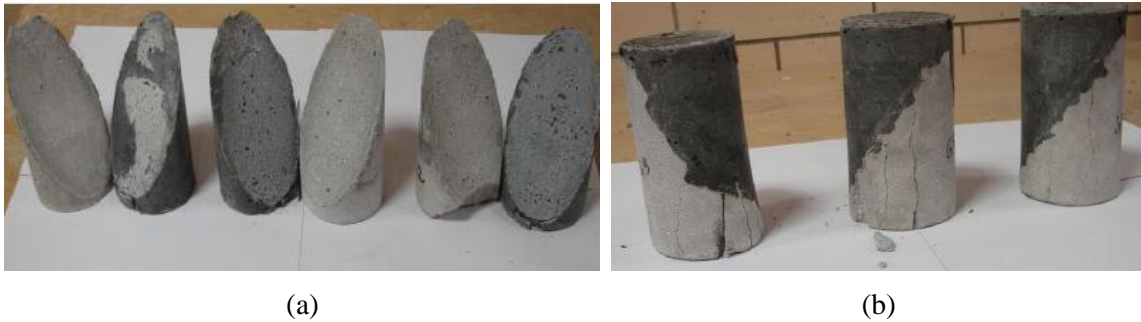
Figure 2.14: Failure Modes; (a) Failure along Interface Plane, (b) Normal Concrete Failure (Harris et al. 2011)
