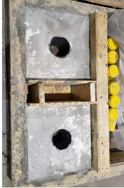
Figure 4.011: Concrete Section of Double Shear Push-off Test Specimen
