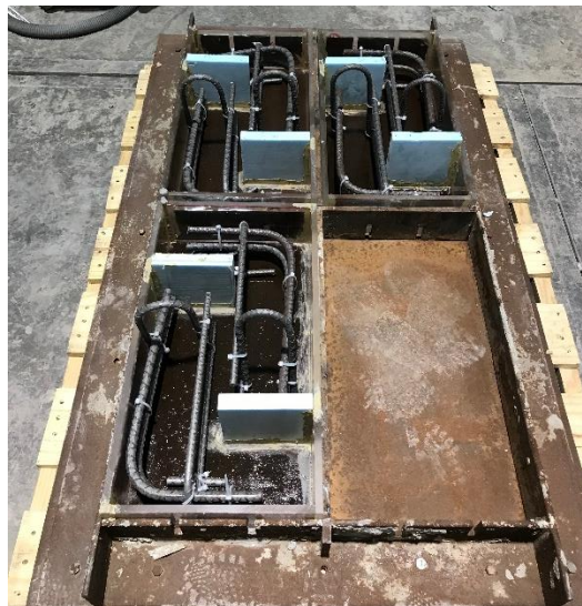
Figure 4.05: L-Shape Push-off Specimen Preparation.
