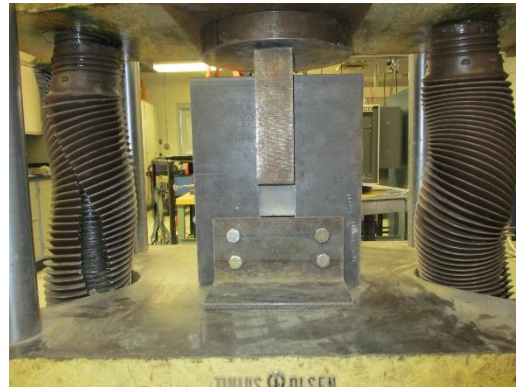
Figure 4.01: Direct Shear Test Setup.
