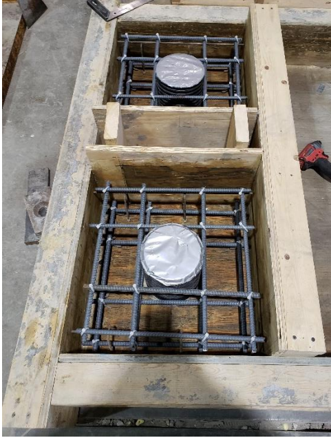
Figure 4.011: Concrete Section of Double Shear Push-off Test Specimen
