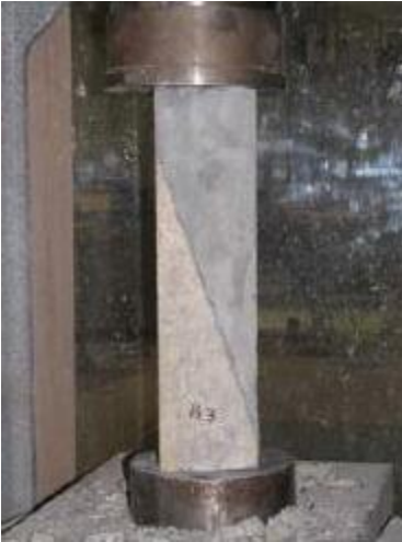
Figure 2.20: Slant Shear Test Configuration (Muñoz 2012).
