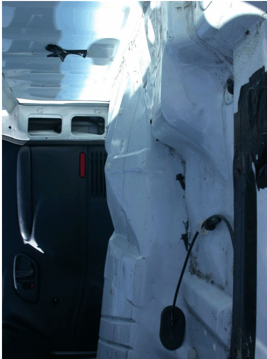
Figure 41. Occupant Compartment Damage, Test NIT-1
