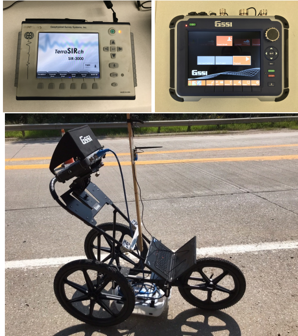
Fig. 1.3. GPR equipment at UNL NDT laboratory
