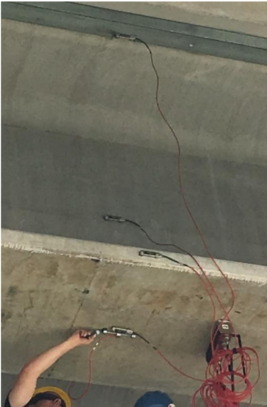
FIGURE 3.4 Installing strain gauges (left) and deflection gauges (right) at the middle section
