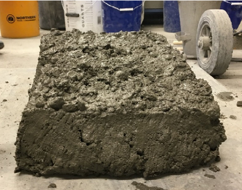
e) 4b-failed edge quality (abundance of excess paste)
