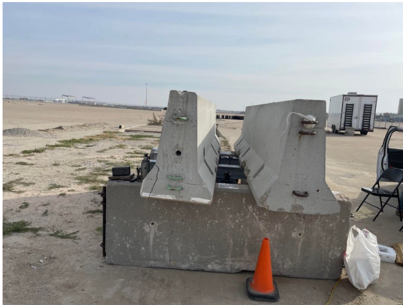
Figure 4.23 A photo of the axial loading test setup with the reaction beam (side view).
