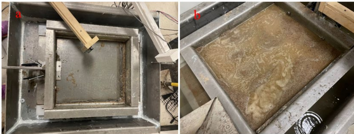
Figure 3.11 Implementation of the large-scale direct shear tests in (a) dry, and (b) submerge conditions.
