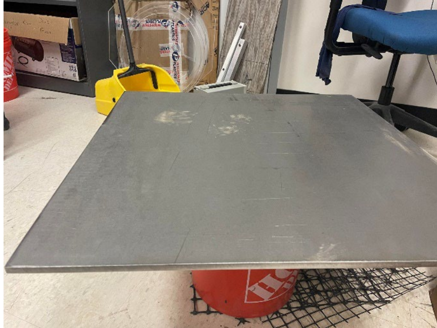
Figure 3.3 The sample of steel plate for large-scale direct shear test.
