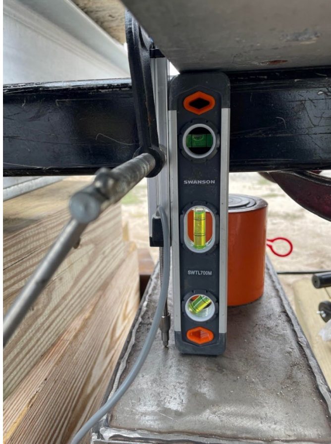
Figure 4.24 The vertical LVDT installed on the top of the bearing plate.
