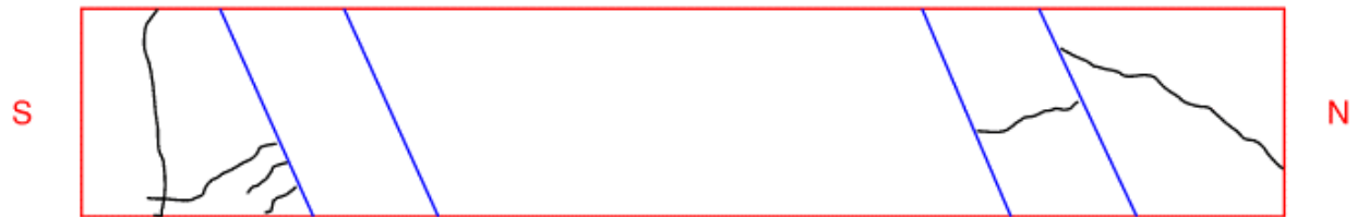
Figure 3.7: Cracking map of approach slab and paving section of Turkey Creek bridge
