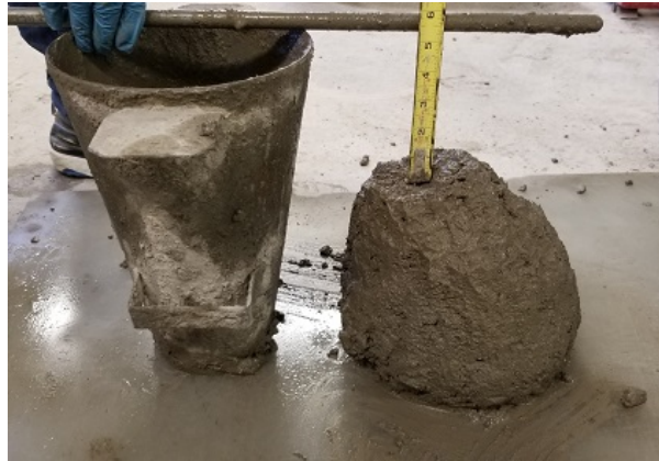
Figure 31. Slump test setup
