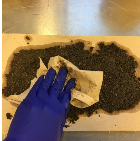
Figure 9. The process of bringing LWFA to SSD condition by a brown paper towel method
