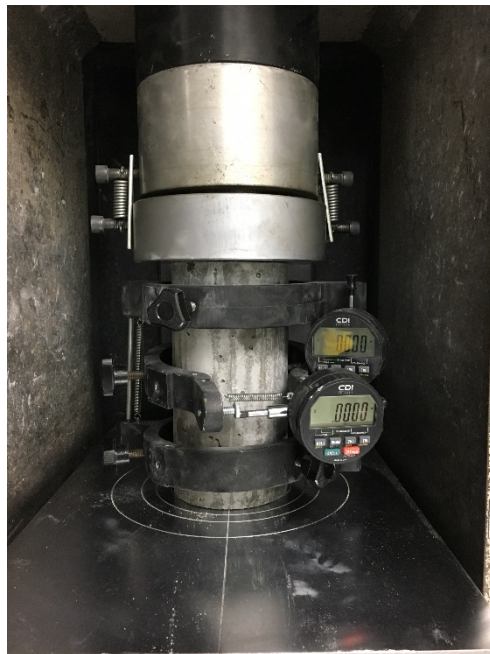
Figure 36. Static Modulus of Elasticity test setup
