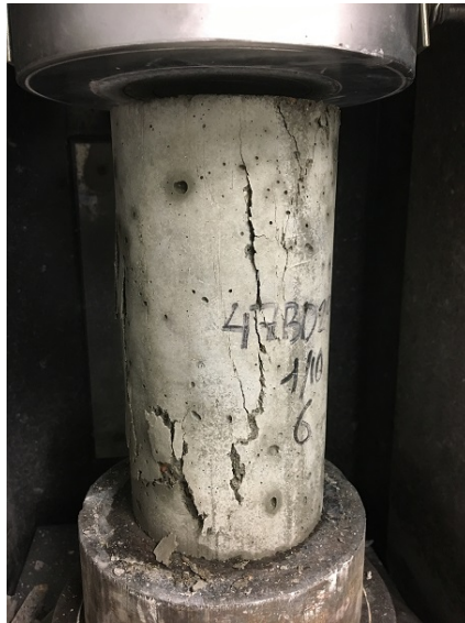
Figure 34. Setup of compressive strength test
