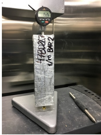
Figure 39. Setup of a free shrinkage test
