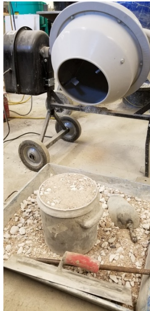
Figure 30. Combined void content test setup
