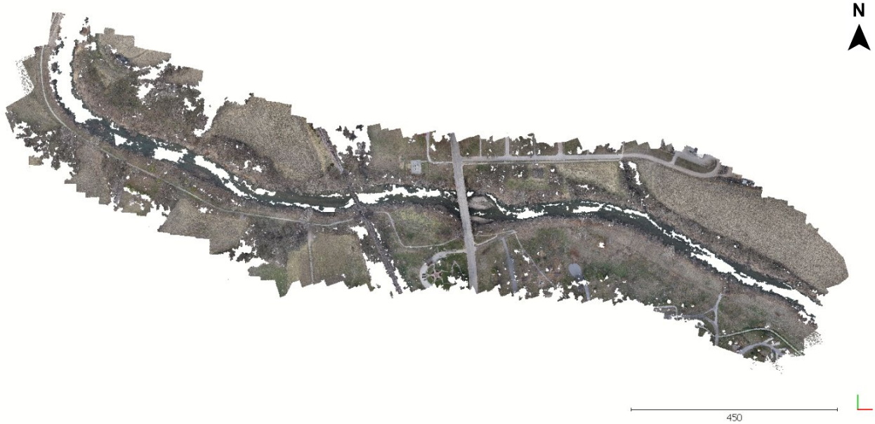
Figure 3.20: Beatrice UAS point-cloud overview (approximately 2100 meters, 6890 feet).
