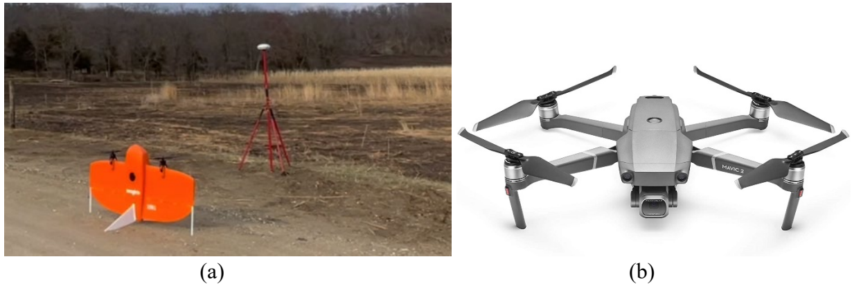
Figure 3.12: PPK-UAS survey: (a) Wingtra and (b) DJI Mavic Pro 2 (DJI, 2022).
